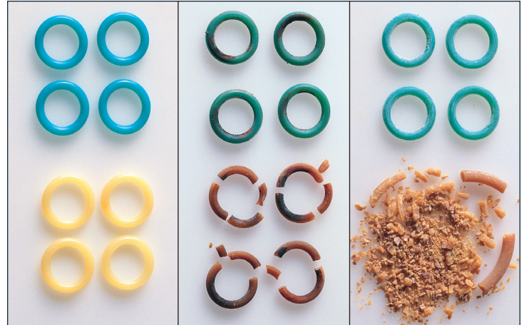
From left, aqua proprietary Resilon® 4301 polyurethane seals and competitor's yellow conventional urethane seals as manufactured; after 1493 hours of exposure to 212°F water; and after 1493 hours of exposure to steam.
