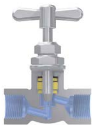
Valve open position
