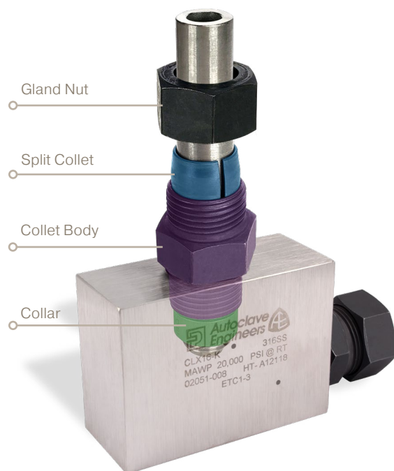
Image 6. Parker Autoclave Engineers cone and thread fitting with anti-vibration collet gland assembly - the collet enhances structural strength and prevents rotation.
